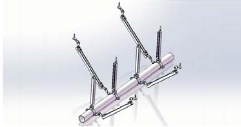
The seismic and dynamic requirements for non-structural installations, such as pipe installations, are often underestimated in comparison to those of structural installations. But even here, the rule is that the weakest link in the chain can lead to failure or to damage.
