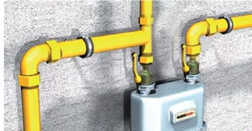
**A specification for the usable anchors emerged from the DVGW-TRGI revision in 2008. This is regulated in TRGI 2008 in Chapter II under item 5.3 "Preparation of pipe installations". In the TRGI from 2008, plastic anchors are now explicitly allowed under certain conditions.**
